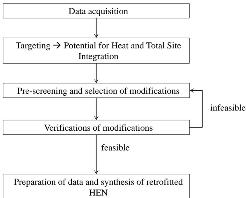
**Figure 1 Methodology used for Heat and Total Site Integration**
