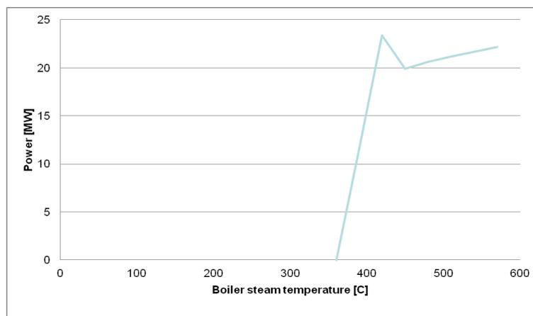
**Figure15 Relationship between Boiler Steam Temperature and Power Estimation**
