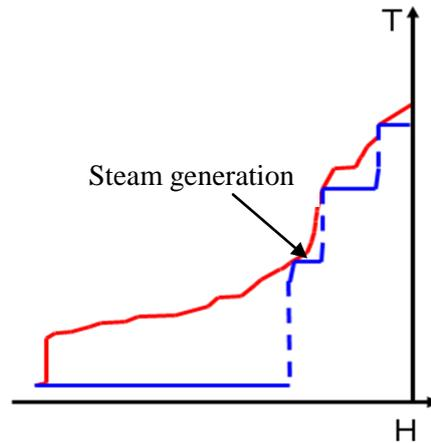
**Figure 8 Site Source Profile and Target of Steam Generation**
