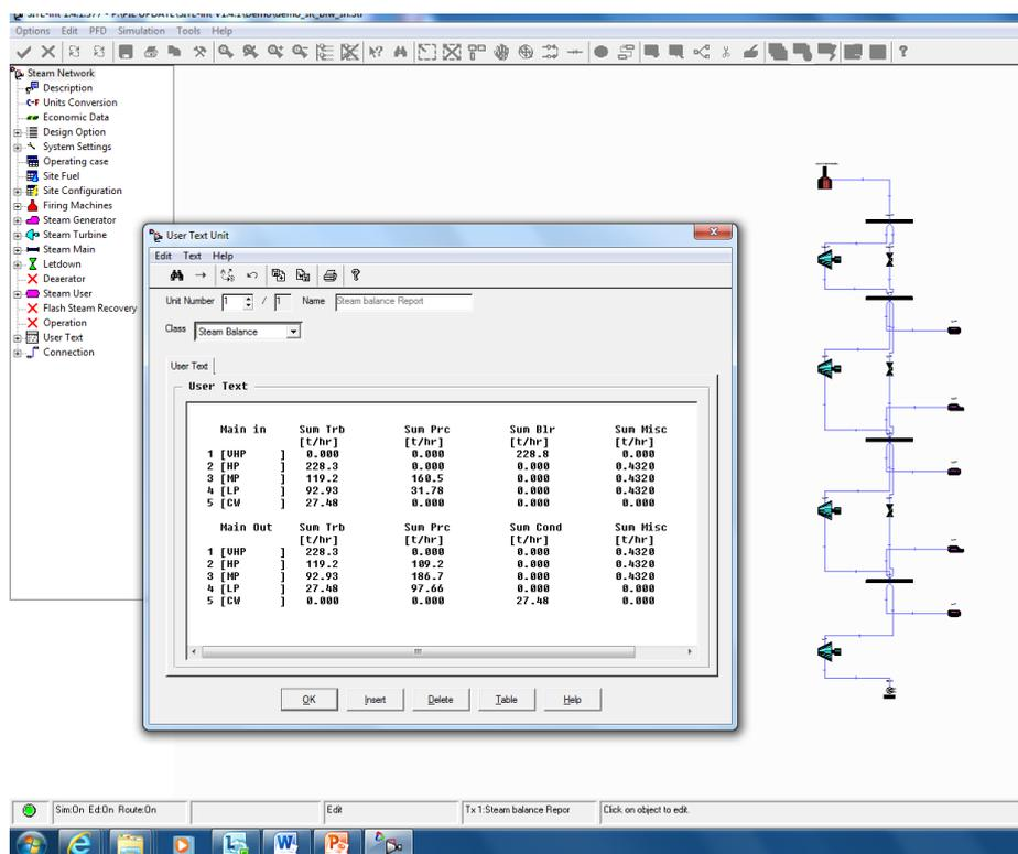
**Figure 17 Site Power Target Estimation using Software ‘EFENIS-Site’**
