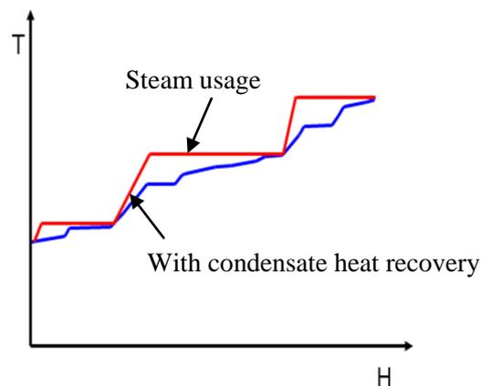
**Figure 11 Site Sink Profile and Steam Usage with Condensate Heat Recovery.**
