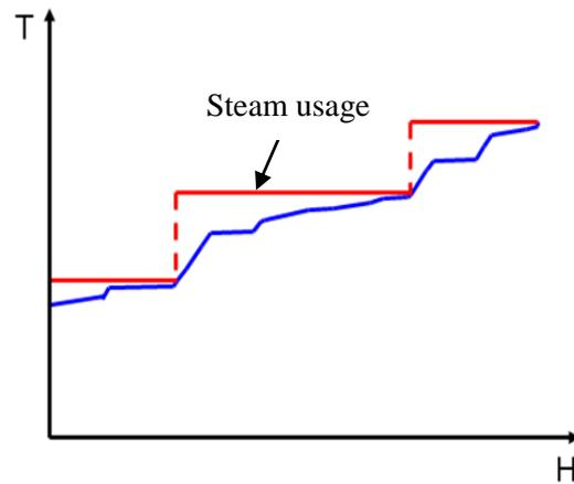
**Figure 10 Sink Profile and Target of Steam usage with Steam Desuperheating**
