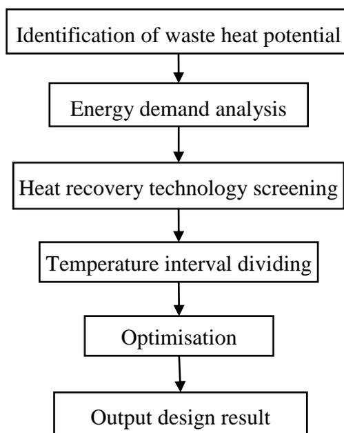
**Fig. 9.** Design flowsheet of waste heat recovery.
