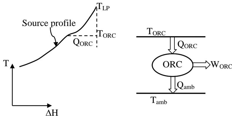
**Fig. 4.** Organic Rankine cycle (ORC) by use of low-grade waste heat.
