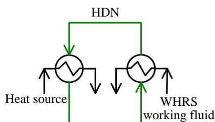
**Fig. 2.** Heat distribution network (HDN) transferring heat between heat source and WHRS.
