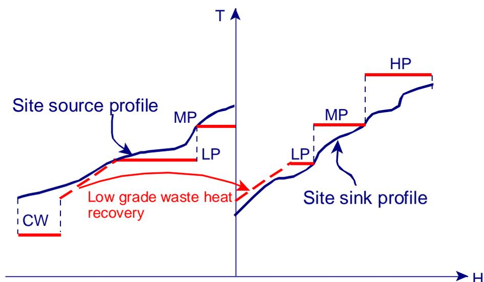
**Fig. 1.** Low-grade waste heat recovery using heat transfer medium runaround.
