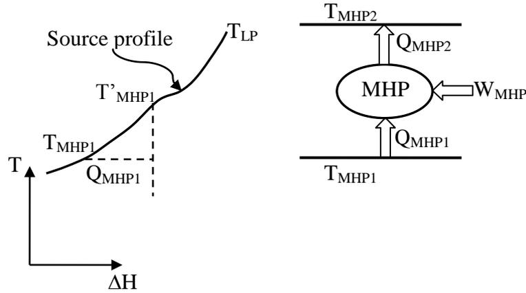
**Fig. 6.** Mechanical heat pump (MHP) by use of low-grade waste heat.
