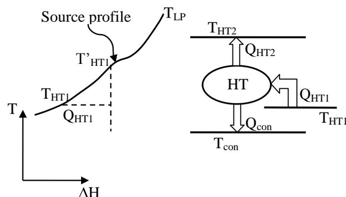
**Fig. 7.** Absorption heat transformer (AHT) by use of low-grade waste heat.
