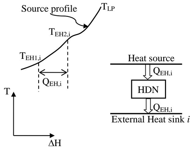
**Fig. 8.** External heating (EH) by use of low-grade waste heat.
