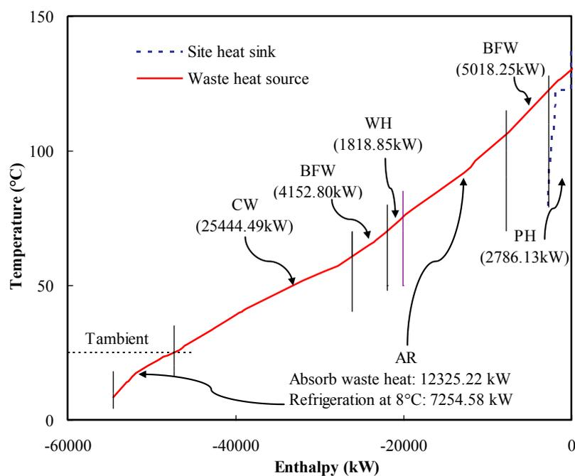
**Fig. 13.** Waste heat recovery design.
