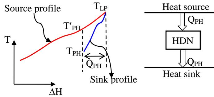
**Fig. 3.** Process heating (PH) by use of low-grade waste heat.
