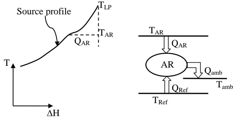
**Fig. 5.** Absorption refrigeration (AR) by use of low-grade waste heat.
